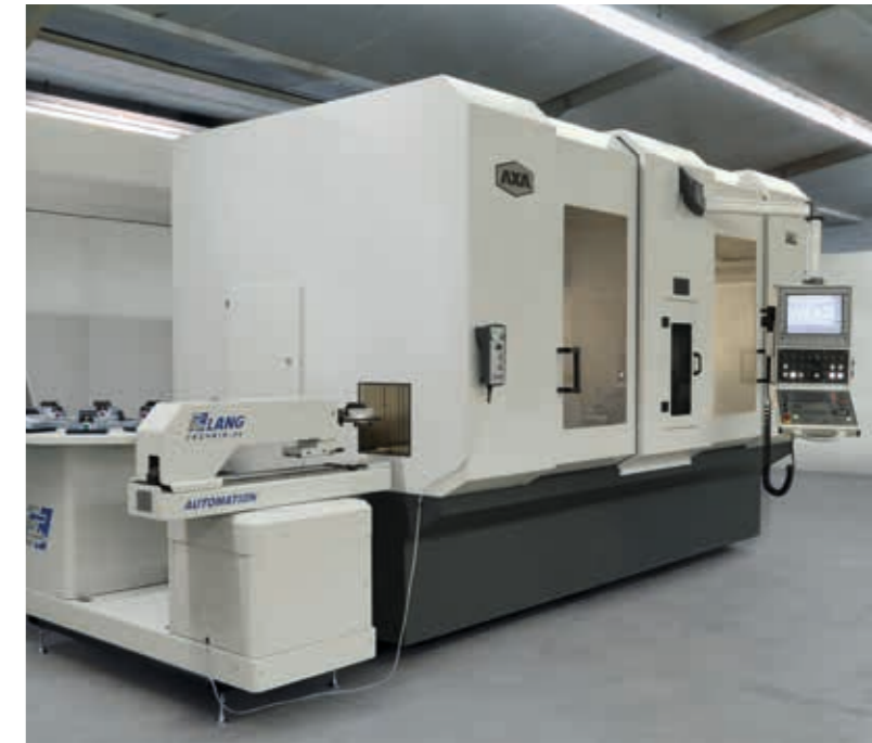
Quick and simple automisation by compact complete solution with workpiece storage, handling system and zero-point clamping
