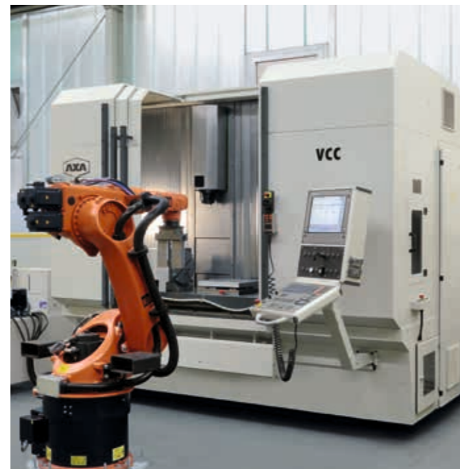
Installed industrial robot in front of the travelling column machine for direct machine loading and unloading with workpieces
